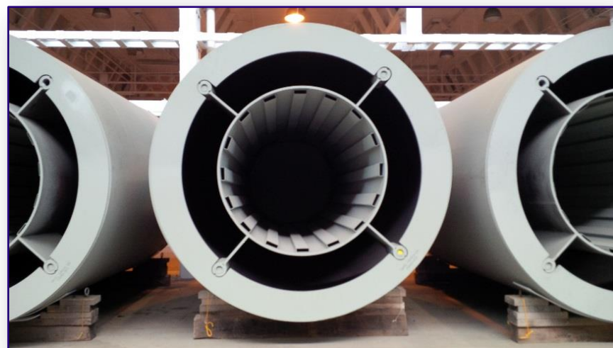
Side View of HI-STORM Overpacks being prepared for Transport
